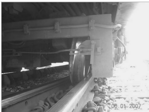
Fig. 3. The derailment resulting from the broken axle in the accident in Istanbul Esenler train station, 2007.
